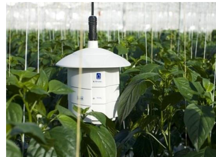
An aspirated thermocouple (thermometer) measures air temperature.
